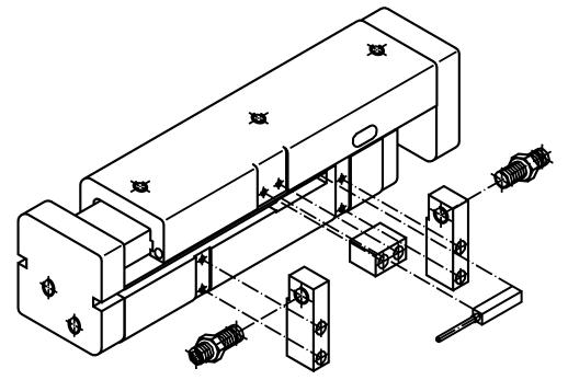
The pneumatic cylinders of type C can be supplied with external and adjustable fixed stops or with small hydraulic shock absorbers.
