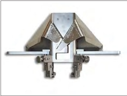
Fig.: edge embossing at a rectangular forming collar
