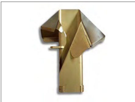
Fig.: loverlap seam on left bag edge for edge folding
